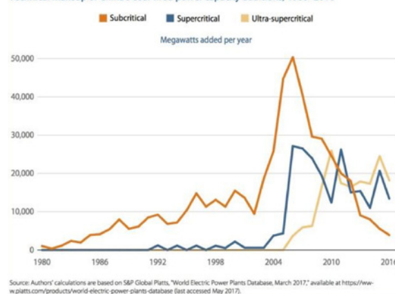
FIGURE 3 China's shift toward cleaner coal-fired power technology Technical makeup of China's coal-fired power capacity additions, 1980–2016
